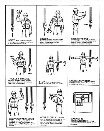
(3) The following hand signals must be used for derricks and a copy must be posted in the cab at the operator's station.
