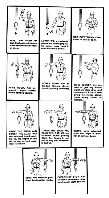
(4) The following hand signals must be used for portal, tower, and pillar cranes and a copy must be posted in the cab at the operator's station.
